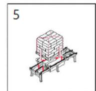
5. The film is slowly slipped under the pallet, locking pallet and load together.
