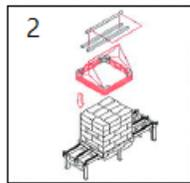
2. Four film grippers move up into the open film.
