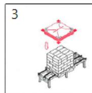
3. Film gripper stretch the completed hood to a size of pallet load.
