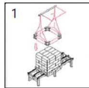
1. Film is opened by vacuum and then retained mechanically.
